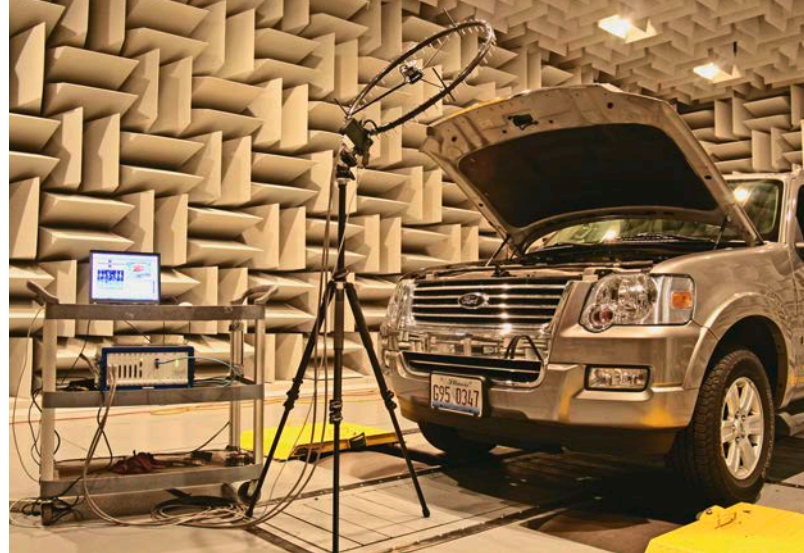
• • • Above: Underhood measurement using a Ring Array. Left: Acoustic Photo 3D of an engine.
