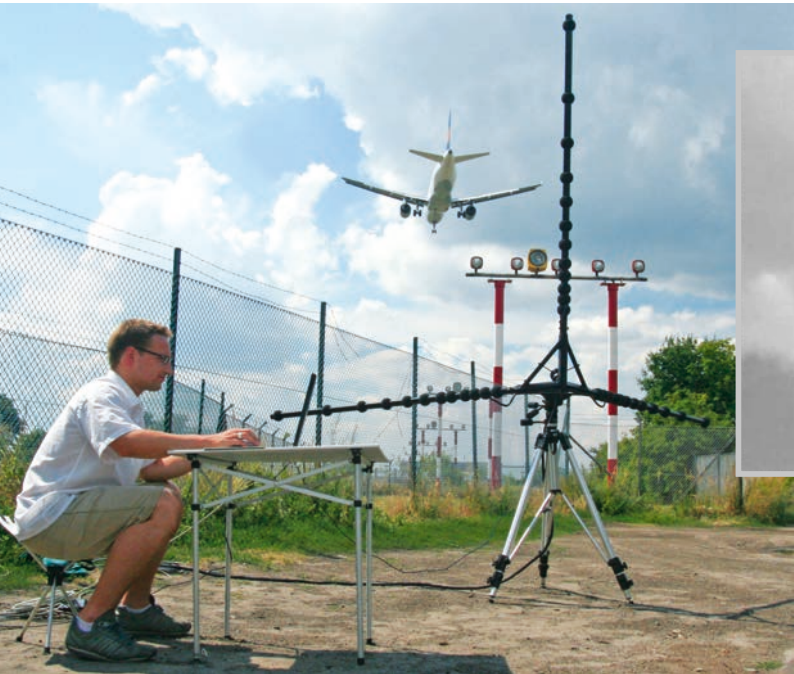
• • • Noise radiation from aircraft engines, gear and flaps and Acoustic Photo 2D.
