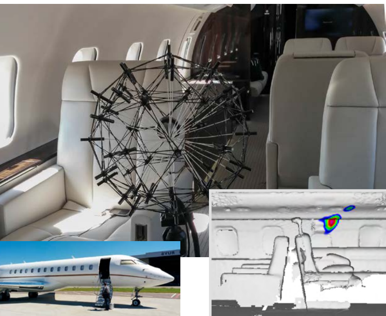
• • • Position of Sphere Array in aircraft cabin and Acoustic Photo 3D.
