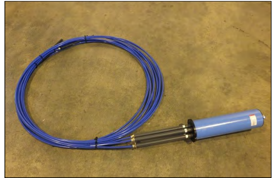
Flexible GEO-XB2 Rod Extensometer fitted with groutable anchors
