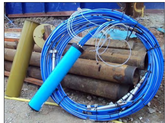
Flexible GEO-XB2 Rod Extensometer fitted with Borros hydraulic anchors
