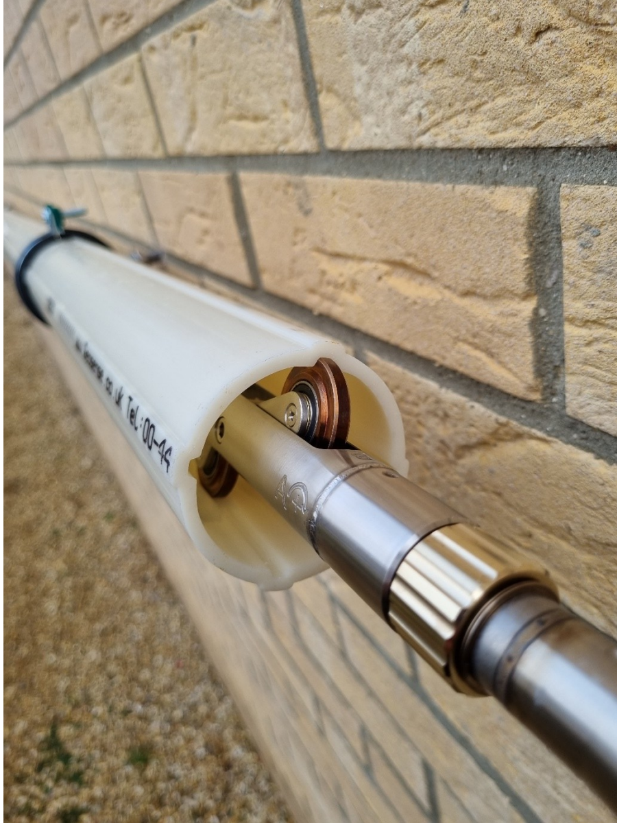
Figure 21: Inclinometer probe inserted into access casing.
