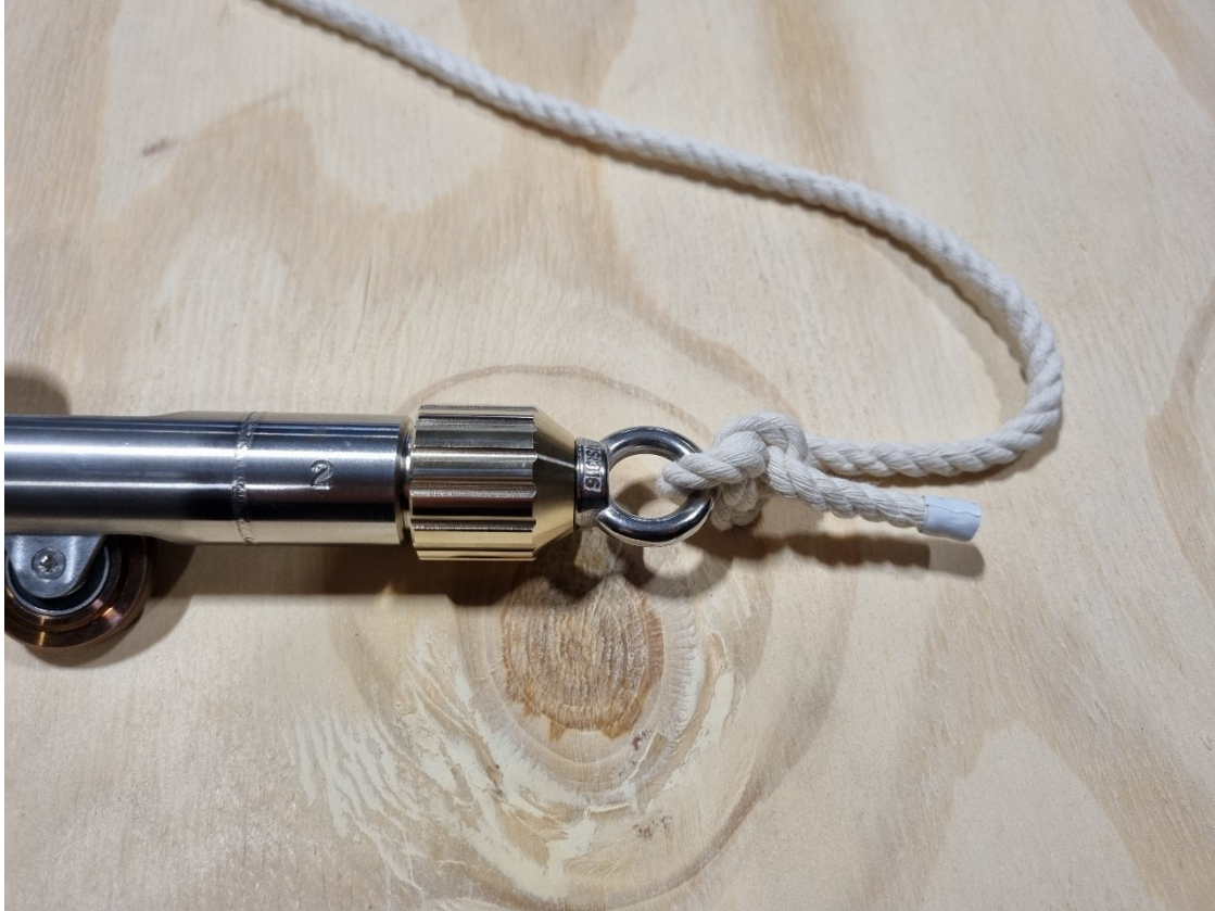
Figure 18: Eyelet cap attached to second end of the probe, marked with 2 rings in later models (a 2 is shown in this model)
