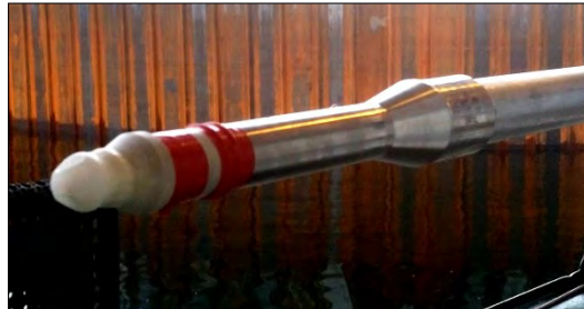
Push-in adaptor for BSP pipe or CPT rods
