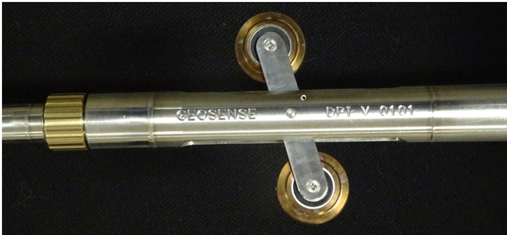
Figure 4: Geosense® Inclinometer Markings
