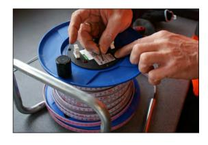
MAKE SURE THAT NO CABLES ARE TRAPPED WHEN REPLACING THE REEL PLATE.
