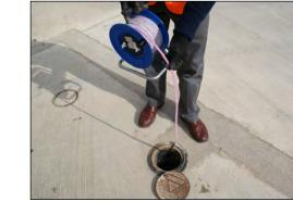
Step 4: Continue to lower the probe until it reaches the bottom of the access casing. As the probe passes through each magnetic target an audible sound (beep) will be heard.
