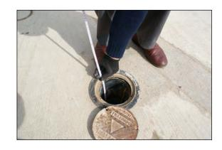
**Step 8:** Without moving your thumb, lift the tape up to read the length
