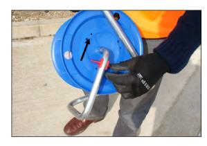
Step 2: Remove the probe from the probe holder.
