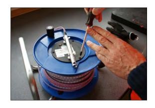
**Step 13:** Remove the old 9V battery and remove the Velcro backing.
