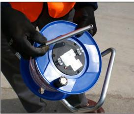
**Step 3:** Slowly lower the probe down the GXM access casing.
