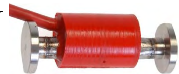
Fig 4. 75mm Embedment Strain Gauge
