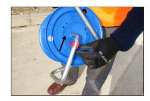
**Step 2:** Remove the probe from the probe holder.
