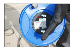
**Step 5:** Lift the probe up until the audible sound (beeping) stops.
