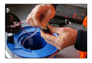
**Step 15:** Attach the new battery and secure onto the Velcro inside the reel
