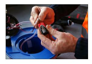
**Step 14:** Apply the Velcro to the back of the replacement battery.
