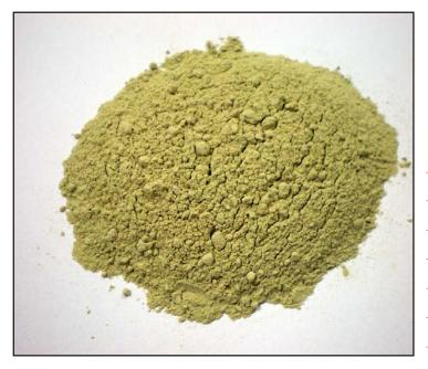
Grout Mix is a pre-blended powder mixture of premium grade high quality sodium carbonate activated Bentonite powder and Ordinary Portland Cement (CEM 1) in a ratio of 2:1.
