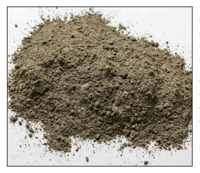
Ordinary Portland Cement (OPC) can be mixed with ballast, sand and gravel for concreting or, together with Bentonite, for grouting.
