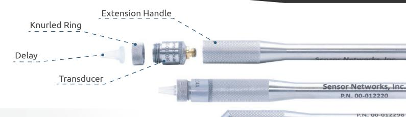
**Pencil probes** are high-frequency, delay-line transducers designed for applications requiring a very small contact face, such as curved turbine blades, spot welds, or thickness measurement from the inside of a pit. They can be used with most flaw detectors and precision thickness gauges and enable the ability to measure down to 0.006" (0.15 mm).
