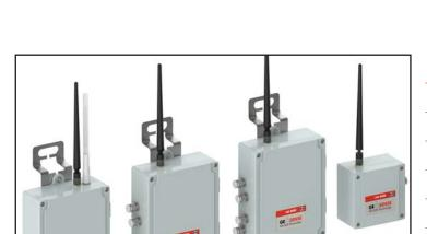
The Wi-SOS MeshNET is a 2.4GHz band, wireless mesh network consisting of a series of wireless Nodes and a Gateway. The Gateway collects the data from the Nodes, stores it locally and it is available to send data to the clouds via 4/3/2G, WiFi wirelessly or via wired Ethernet, RS485. All the data is displayed via the Web Port, where customer data can further be viewed and downloaded locally via .csv, remotely via SFTP/FTP or programmably via API.
