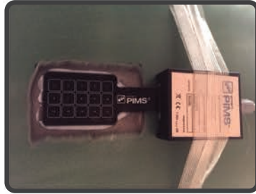
matPIMS™ 3x5 matrix permanently installed with RS-485 cable back to surface for data collection, pre-overwrap.
