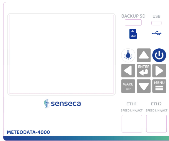
Fig. 6.1: Display & keyboard for MTD-4000
